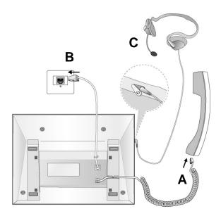
A Connect the telephone cord (spiral cord) to the handset and the other end to the handset jack at the bottom of the telephone.
