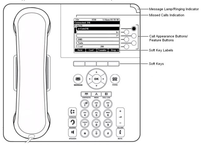
This phone supports 24 programmable call appearance/feature buttons. The labels for 6 of these buttons are visible on the main display and can be controlled by the adjacent buttons to the right. You can use the ▲ up and down ▼ arrow keys to scroll the display. You can also use the ◀ left and right ▶ arrow keys to move through the button features in pages of 6.
