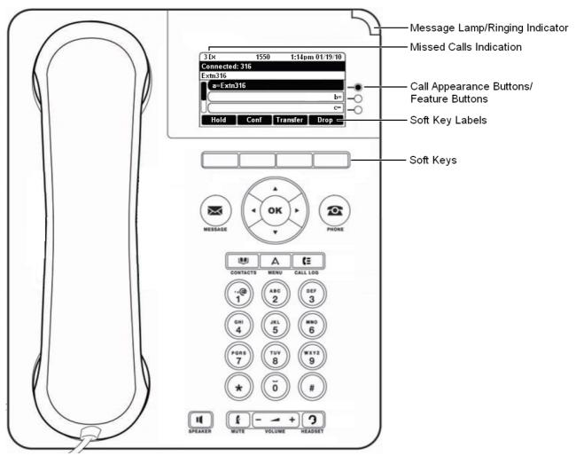
This phone supports 12 programmable call appearance/feature buttons. The labels for 3 of these buttons are visible on the main display and can be controlled by the adjacent buttons to the right. You can use the  $\triangle$  up and down  $\nabla$  arrow keys to scroll the display. You can also use the  $\triangleleft$  left and right  $\triangleright$  arrow keys to move through the button features in pages of 3.
